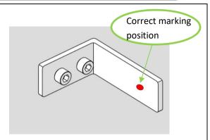
5. Test the position of the brackets by marking them with a drill bit through the pre-drilled pilot holes. The marks should be in the centre of the bracket (top to bottom).
